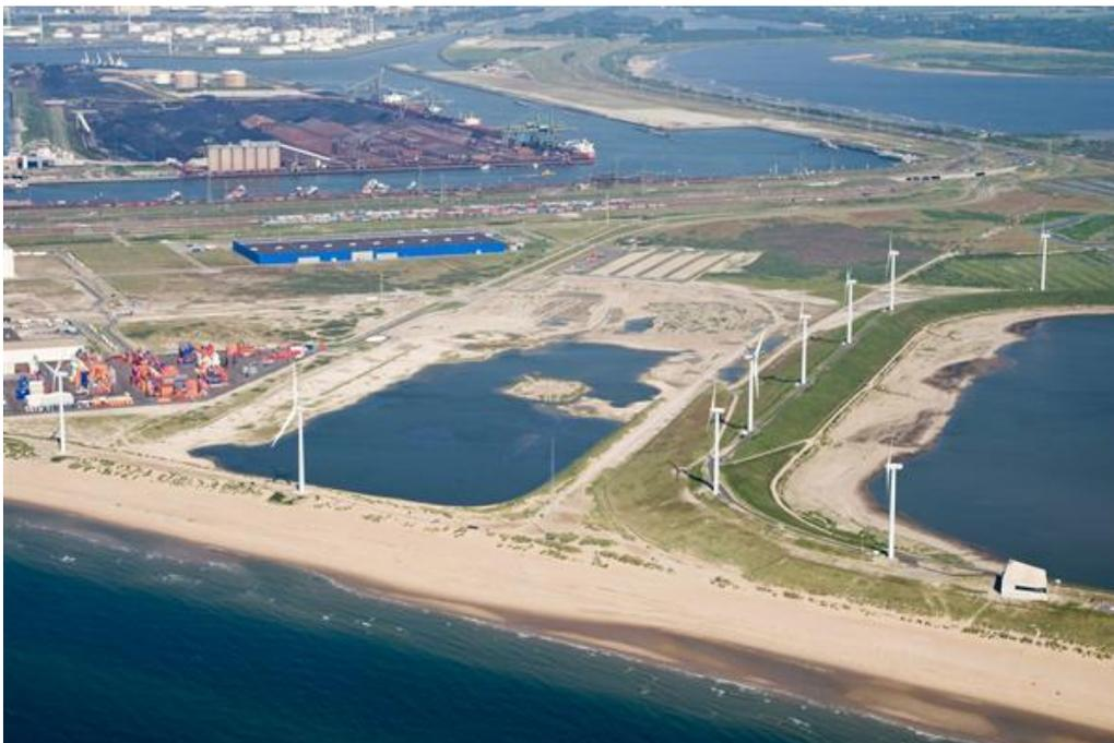
Figure 1 Slufter (right of the wind mills) with desanding basins on the left of the mills (no longer used). Unloading is in the bend of the harbour (Hartelhaven), 2 km from the Slufter.
